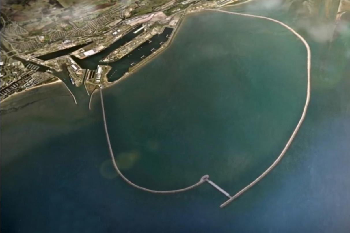
Figure D4: Artistic impression of a future tidal lagoon power plant, where an artificial lagoon is created within seawalls
